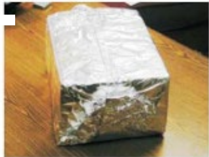
The finished foil wrapped sample should be tightly sealed on all sides.
